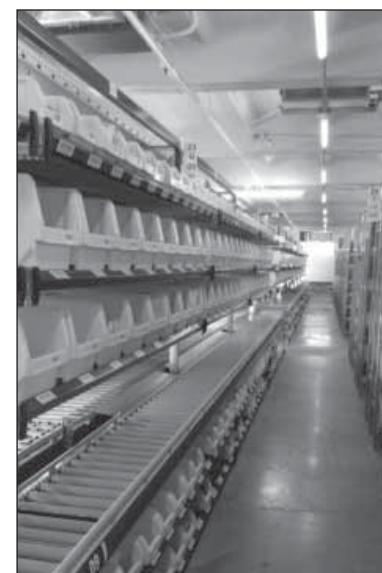
A gravity flow racks structure at a pharmaceutical warehouse
